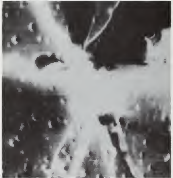
FIGURE 16. SCANNING ELECTRON MICROGRAPH OF THE FRACTURE SURFACE AT A FLAW OF A TENSILE SPECIMEN; EPON 828 + 10 pph CTBN 20-64 (SMALL PARTICLES) + 5 pph CURING AGENT D.
